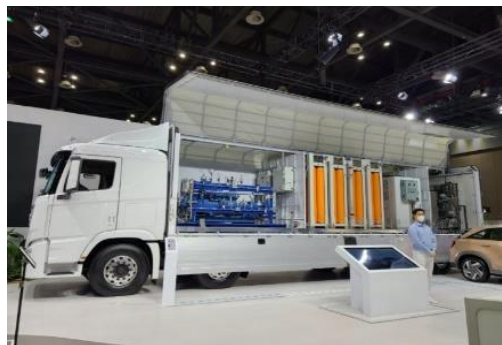
Mobile Refueling Station
