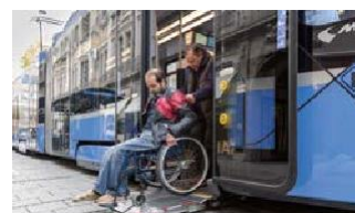
A wheelchair lift enables passengers with reduced mobility to board the train without barriers, even from street level.
